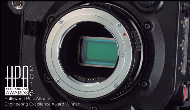
Super 35 mm Imager and EF Lens Mount*
