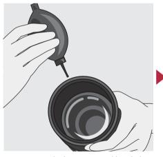
First, remove the lens cover and brush the dust from the lens surface with a soft brush or blower brush.
