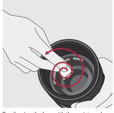
Gently wipe the lens with the moistened lens paper in a circular motion, from the center to the edges. Take a dry piece of lens paper and wipe until all smears disappear.
